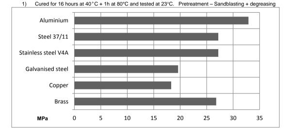
Average lap shear strengths of typical metal-to-metal joints (ISO 4587) (typical average values)
