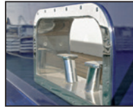
Stainless steel bracket in aluminium shell plate
